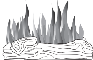
Figure 34 - Incorrect Burner Flame Pattern When Using Wrong Gas Type
