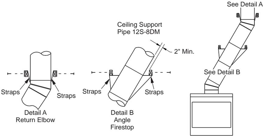
**Figure 10 - Ceiling Support Pipe 12S-8DM**
