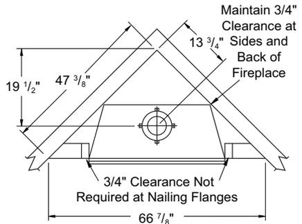
Figure 2 - Corner Installation
