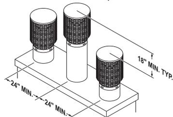
**Figure 18 - Multiple Chase Installation**
