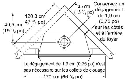
Figure 2 - Installation en coin
