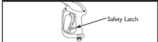
Figure 8 — Spray Gun with Safety Latch Engaged
