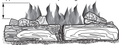
Figure 26 - Correct Burner Flame Pattern
