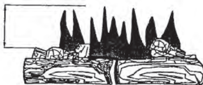
Figure 20 - Incorrect Flame Pattern with heater set to High Flame
