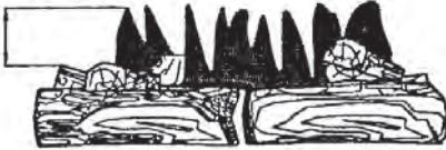
Figure 19 - Correct Flame Pattern with heater set to High Flame
