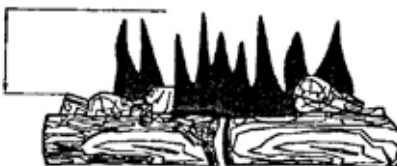
Figure 27 - Incorrect Flame Pattern with heater set to High Flame
