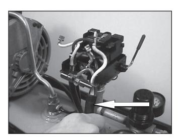
2. To change out pressure switch, first remove the pressure relief tube using an adjustable crescent wrench. With the same wrench, remove the pressure switch from the manifold. To re-assemble, repeat these steps in a reverse order.
