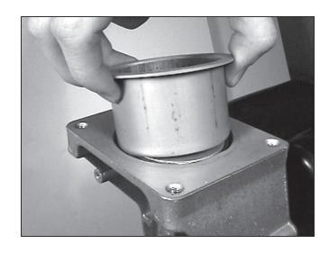
17. To change the eccentric/bearing assembly, simply loosen the counter balance screw with a 3/8" nut driver and slide it off the motor crank.
