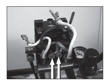
d. To take out the cord assemblies, loosen the bracket bar with a 5/16" nut driver. Slide out the cords from the bottom.
