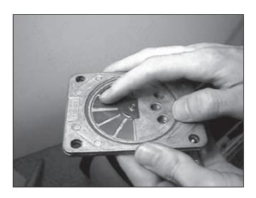
15. To replace the fan, you will need the 3/8" nut driver. Hold the fan while unscrewing the fan bolt and washers. The fan will then slide off the eccentric/bearing assembly.
