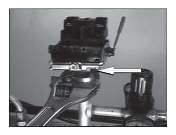
3. If the gauges are faulty, use the 7/16" crescent wrench to remove them from the regulator. When screwing the new ones on, be sure to put the tank gauge on the right and the regulator gauge on the left.
