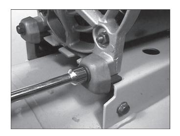
19. When reapplying the eccentric/bearing assembly, only push it far enough on the motor crank to get it even with the tip of the crank. Torque the eccentric bolt to 100 to 120 in.-lbs.
