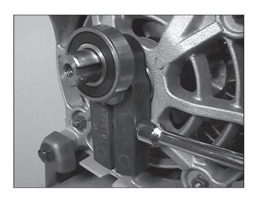
18. With all of the compressor components removed from the motor assembly, the motor can easily be removed by unscrewing the foot bolts with a 3/8" nut driver and sliding the motor, in the proper direction, off the frame clip.
