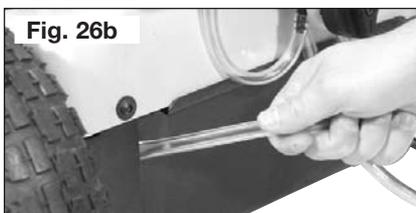
3. Place end of cleaning solution hose into a suitable container to drain cleaning solution. (See Fig. 27)
