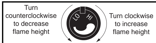
Fig. 20 Flame adjustment knob for Honeywell Valve.
