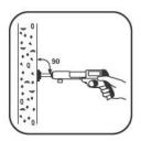
1. ALWAYS hold tool perpendicular to work surface.
