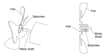
Figure 7 - Fan, Motor Shaft, and Setscrew Location
