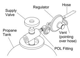
Figure 3 - Regulator With Vent Pointing Over Hose
