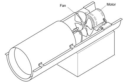
Figure 6 - Fan Removal
