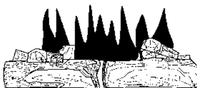
Figure 16 - Incorrect Flame Pattern with Control Knob Set to High Flame
