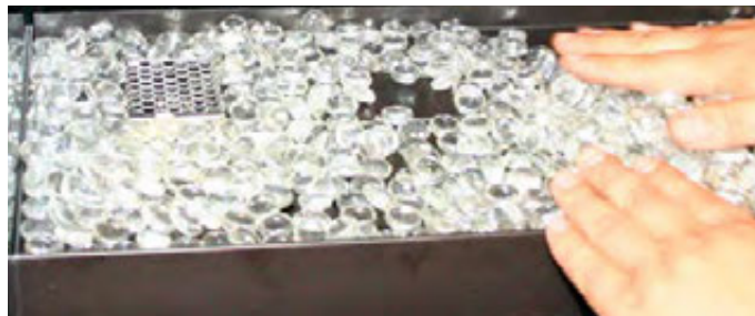
Figure 24. Installation of the firestones. (Ensure ONLY one layer of firestones cover the surface).
