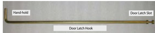
Figure 23a. Door buckle Tool
