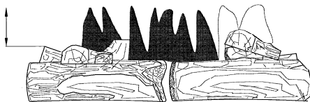
Figure 29- Correct Flame Pattern with Control Knob Set to High Flame (5)
