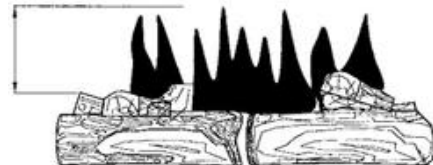
Figure 30 - Incorrect Flame Pattern with Control Knob Set to High Flame (5)
