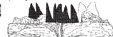
Figure 17 -Correct Flame Pattern with Control Knob Set to High Flame
