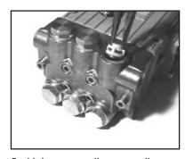
2. Using a needle nose pliers, remove the inlet and discharge valve assemblies (#32X).
