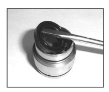
12. Use a flat screw driver to pry the oil seals (#19) loose from the seal case (#20).
