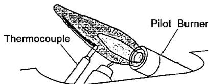
Figure 23 - Correct Pilot Flame Pattern
