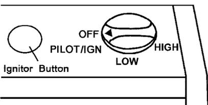
**Figure 16 - Control Knob In The OFF Position (KWN111)**
