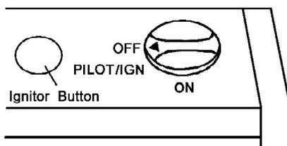
**Figure 15 - Control Knob In The OFF Position (KWN109)**
