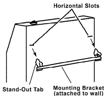
**Figure 10 - Mounting Heater Onto Mounting Bracket**
