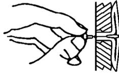
**Figure 9 - Popping Open Anchor Wing For Thin Walls**
