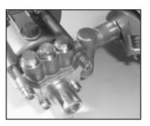
With a crescent wrench, remove the injector retainer (47). Inspect the o-ring (46) for wear and replace as necessary.
