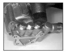
Tap the back of the manifold (35) with a rubber mallet to dislodge, and slide off the plungers. (8). Take note of the position of the discharge port so as to place the manifold in the same position during reassembly.
