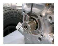
Using a 5/32" allen wrench, remove the set screw holding drive gear onto engine crankshaft.
