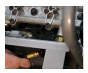
Pull pulse hose underneath the frame from the rubber mounting grommet, so the hose will hang free.
