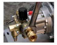
Screw quick connect fitting onto chemical injector.
