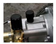
Install black oil plug in top of pump before attempting to start and run pump. Your new Giant GXH2525A-112H pump has an adjustable unloader valve with bypass. You will need to turn the Black knob clockwise to increase your new pump to maximum pressure.
