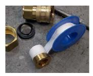
Apply Teflon tape to threads of inlet nipple Note: for model XC2625 you will need to install the 90 Degree fitting part # 2103 to allow the water supply line adequate clearance to be attached properly.
