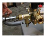
Insert nipple through nut, and thread the nipple into the pump head. Tighten with a 1/2" allen socket.
