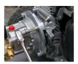
Using a 5/16" allen socket, screw the four mounting bolts through the pump, into the flange. Snug. \*Recheck these bolts after 2 hours of running time.
