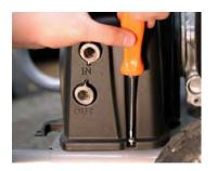
Remove the two Phillips head screws holding the plastic shroud in place
