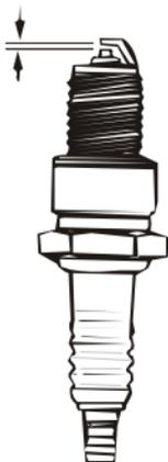
5. Install the spark plug carefully, by hand, to avoid cross-threading.
