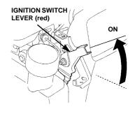
Some engine applications use a remotely-mounted ignition switch rather than the engine-mounted ignition switch shown here.
