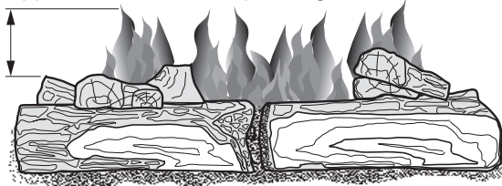
Figure 31 - Correct Burner Flame Pattern
