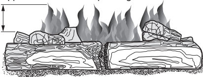
Figure 30 - Correct Burner Flame Pattern
