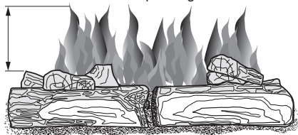
Figure 31 - Incorrect Burner Flame Pattern
