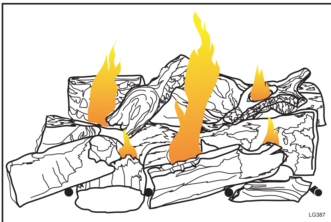
Fig. 58 Correct flame appearance for DVBR42 model.
