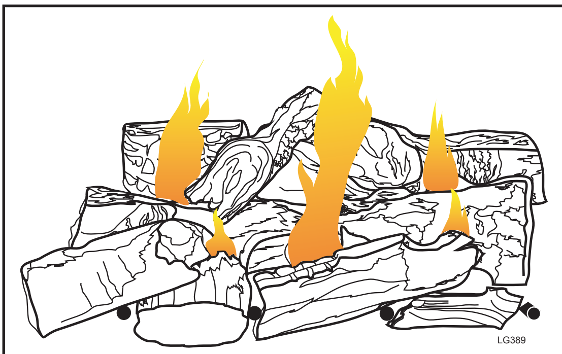
Fig. 57 Correct flame appearance for DVBR36 model.
