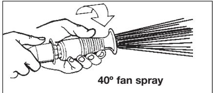
For low pressure operation, extend the nozzle of the multi-adjustable spray wand as shown.
