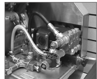
Giant (beltdriven) P316 (unloader mounted on pump)
