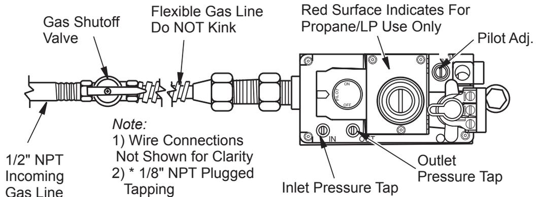
**Figure 18 - Connecting Flexible Gas Line to Millivolt Valve**
