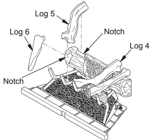
**Figure 24 - Installing Logs 5 and 6**
