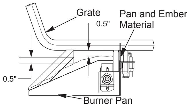
**Figure 21 - Pan and Ember Material Clearances**
