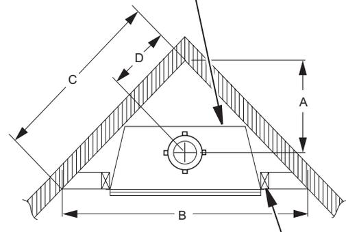
3/4" Clearance Not Required at Nailing Flanges
