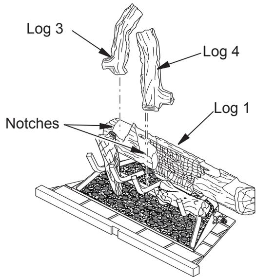
**Figure 27 - Installing Logs 3 and 4**
