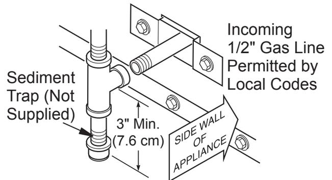
*Figure 17 - Sediment Trap*
