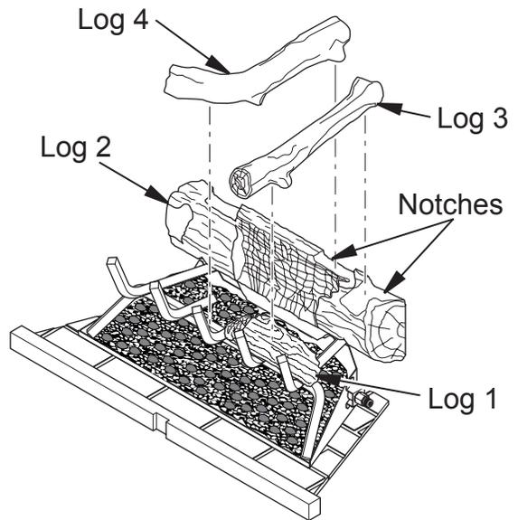
**Figure 23 - Installing Logs 3 and 4**
