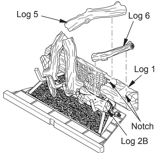
**Figure 28 - Installing Logs 5 and 6**
