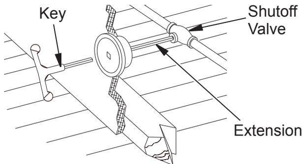
Typical Exterior Wall Gas Shutoff Installation
