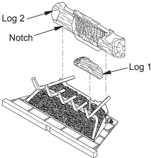
**Figure 22 - Installing Logs 1 and 2**
