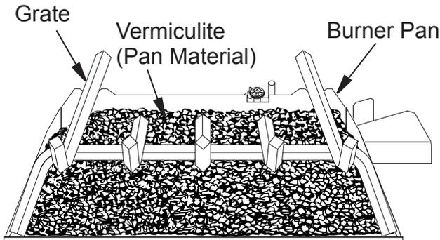
**Figure 19 - Fill Entire Burner Pan with Vermiculite**
