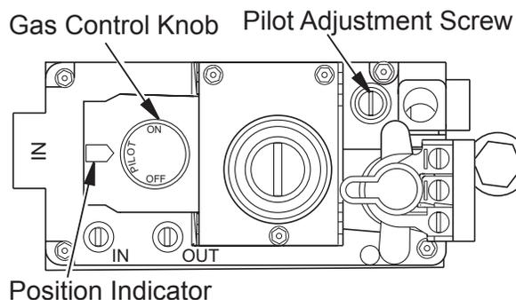
**Figure 36 - Control Knob in the PILOT position**
