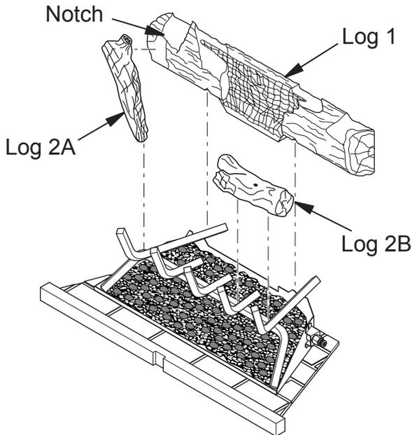
**Figure 26 - Installing Logs 1, 2A and 2B**
