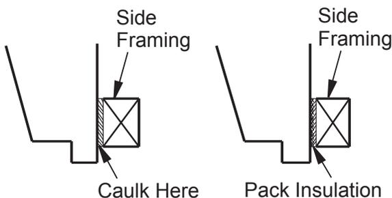
**Figure 31 - Sealing Between Appliance and Framing**
