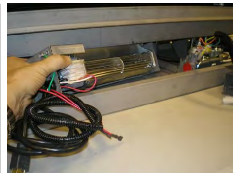
3. Insert fan and place at right rear corner of unit. See Component Locations Section in manual.
