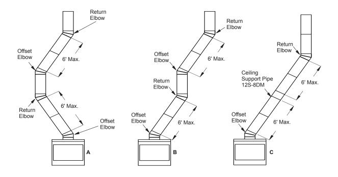
Figure 9 - Typical Offset Installation
