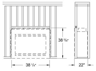
Figure 1 - Framing Dimensions
