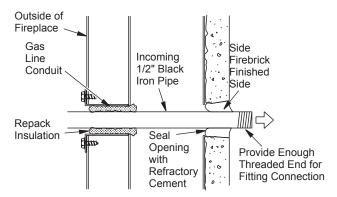
Figure 22 - Gas Line Installation
