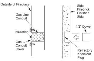
Figure 21 - Gas Line Knockout
