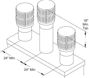
Figure 18 - Multiple Chase Installation
