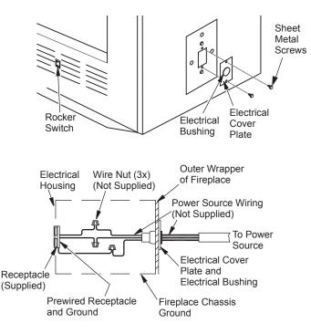
Figure 6 - Fan Switch-Electrical Bushing
