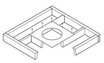
Figure 13 - Firestop Spacer with Attic Space Above Ceiling
