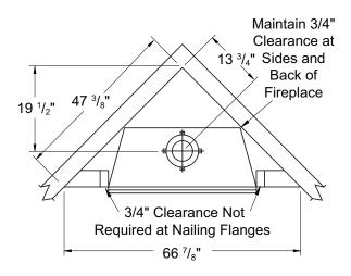
Figure 2 - Corner Installation
