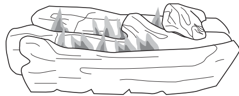
Figure 45 - Correct Burner Flame Pattern
