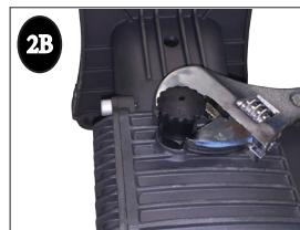
2. Thread in the supplied breather by hand turning clockwise. Use a crescent wrench to fully tighten the breather to the pump.
