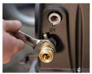
Then use a 7/8" wrench to unscrew the chemical injector/quick connect fitting from the pump.
