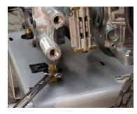
Using a 3/4" wrench, remove unloader valve. This will ease the removal of the pump.
