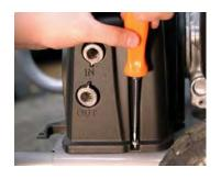
Remove the two Phillips head screws holding the plastic shroud in place
