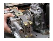
Slide pump off engine shaft. You may have to angle the pump slightly to allow the pulse hose to come out of the hole in the frame.
