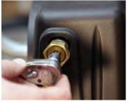
Remove filter from inlet nut, and using a 3/8" allen wrench or socket, unscrew the inlet fitting from the pump.
