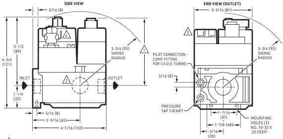
WITH V5306 (ILLUSTRATED), V5307 OR V8305 PRESSURE REGULATOR: 24V MODELS-3-1/2 (89), 120V MODEL-3-5/8 (92) MANUAL MODELS-2-13/16 (71), FOR V5308 ADD 5/8 (16) TO DIMENSIONS GIVEN.
