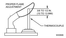
Fig. 13. Proper Flame Adjustment.
