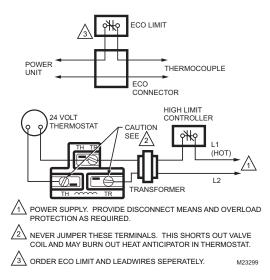
Fig. 9. Typical Wiring Hookup for 24V Systems.
