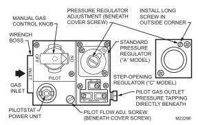
Fig. 6. Top View of Standard Capacity Gas Control.
