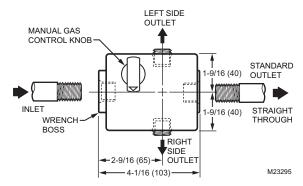
Fig. 3. Optional Side Outlets (Standard Capacity Models only).
