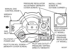
Fig. 7. Top View of High Capacity Model.
