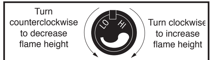
Fig. 25 Flame adjustment knob for Honeywell valve.
