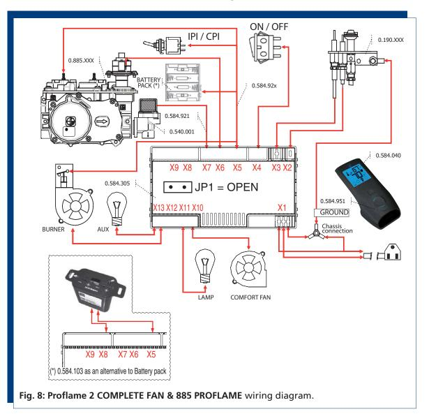
Note: the models of IFC boards that can operate in either ATMO or in FAN mode, are configured in the factory in ATMO mode (Jumper JP1 closed). To enable the FAN mode, it is necessary to open the IFC removing the cover and than remove the jumper JP1 (JP1 open), see Picture and Table below.
