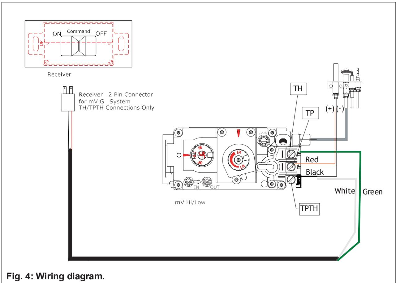
Fig. 4: Wiring diagram.
