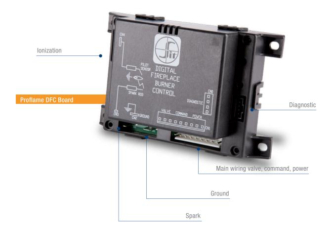
For operation with a less sensitive response time to movement of the flame with relationship to the sensing electrode, the DFC unit can be ordered with extended "FFRT" option (CSA certified only). With this option a "Flame Failure Response Time" (5s) with extended "Recycle Time" (30s) are adopted. In case of flame failure detection, the system will not react immediately, but will wait for FFRT expiration before entering lockout.
