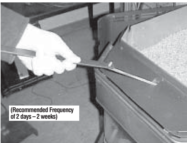
Figure 38 - Pulling Tube Scraper Rod
