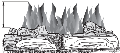
Figure 29 - Incorrect Burner Flame Pattern
