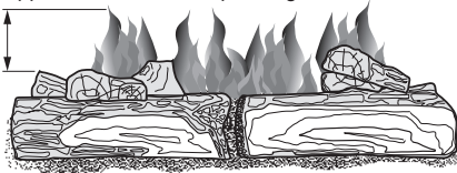
Figure 28 - Correct Burner Flame Pattern
