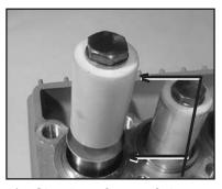
9) Check surfaces of plunger (16). Damaged surfaces cause accelerated seal wear. Deposits of all kinds must be removed from the plungers.
