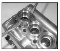
6) Remove seal case (20) and weep return rings (25) from the valve casing.
