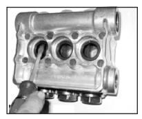
7) Remove the pressure rings (24) and v-sleeves (23 - Note: P422 & P423 pumps have a spacer ring) from the valve casing (26).
