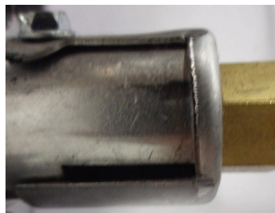
Figure 1 - Air shutter at 1/8-inch opening
