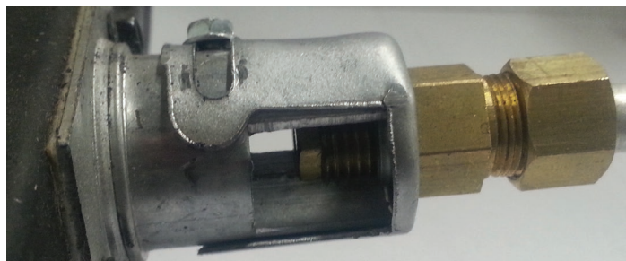
Figure 3 - Air Shutter Fully Open
