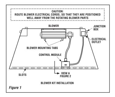
**Step 6.** If electrical power has not been provided to the unit's junction box receptacle - Route a 3-wire, 120Vac power line to the unit's junction box. Remove the receptacle by removing the two securing screws. Connect the supply wires to the receptacle as shown in *Figure 4*. Reinstall the receptacle.
