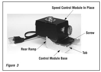
**Step 10.** Place the speed control module base in the lower opening of the firebox (*refer to Figure 2*). Engage the tabs in the slots on the firebox bottom floor front lip. Then place the speed control module on the module base, between the rear ramps. Push the module back, sliding it up the rear ramp of the base, and secure it in place using the provided screw in the hole at the front of the base (*refer to Figure 3*).
