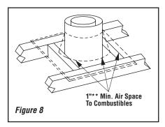
Security's chimney sections do not need to be screwed together. Additional reinforcement is not necessary except in certain offset conditions (refer to *Page 7*, *Figure 22*).
