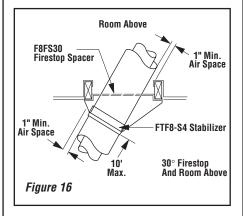
To clear any overhead obstructions, you may offset your chimney system using Security's 30° offset and return elbows. Use two elbows - an offset elbow to initiate the offset and a return elbow to terminate it. A 30° offset elbow, angling in any direction, may be the first component used off the top of the fireplace flue collar.
