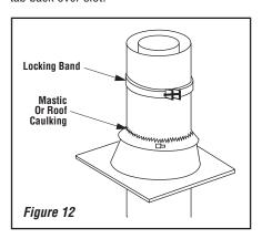
Seal storm collar to outer chimney with roof caulking or mastic around entire circumference of pipe. Also add extra roof caulking to the tab/slot area to seal completely against water penetration (*Figure 12*). Check all joints very carefully to ensure no water intrusion can take place.
