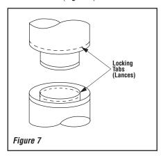
**Note:** Assemble one component of chimney at a time (inner section first, then outer section last) before proceeding with the next complete section.
