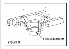
**Note:** Do not apply excessive pressure to any subsequent chimney sections following the stabilizer when installing. Ensure each subsequent chimney section is securely attached by testing as noted in **Step 4**.
