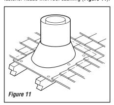
**Step 8.** The standard Security Chimneys FTF8 roof flashing assemblies include a storm collar. Slide the storm collar over outer chimney, rest on flashing spacers and align with top surface of flashing. Insert tab in slot, pull tight and bend tab back over slot.
