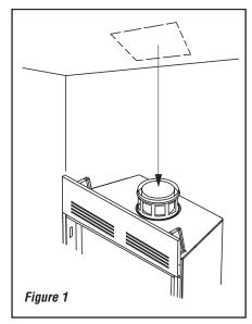
Nail permanently, using at least two (2) more fasteners, after chimney sections have been assembled through the thimble/firestop spacer combination and after any necessary adjustments have been made. Firestop spacer must be secured by at least four (4) fasteners when completely installed.
