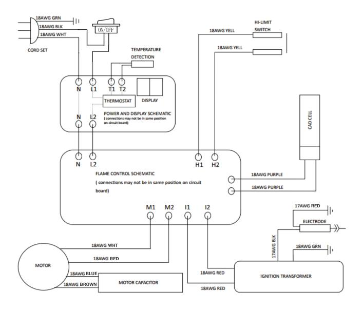
The parts lists and wiring diagram show the heater as it was constructed. Do not use a heater which is different from that shown. Heater performance is effected by air pressure setting. If there is any uncertainty about the air pressure
