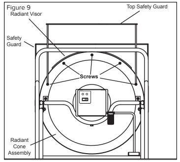
5. Attach top safety guard using the two outer-most extra screws on the top of the radiant cone (see Figure 9).
