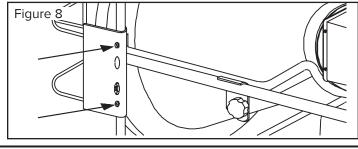
Attach Radiant Visors to the top and bottom rear of the Radiant Cone Assembly using extra screws included.
