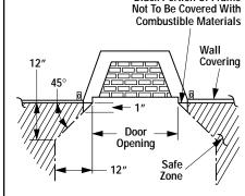
\*Both Of These Dimensions Must Be At Least 18" When An Unvented Gas Log Set Rated At 32,000 BTU Or Higher Is Used. (Maximum 40,000 BTU)
