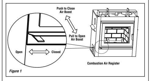
For instance, a long chimney will necessitate closing the damper more. To obtain the proper combustion, close the damper completely, then open it about 1/4" to 1/2" (6.4mm to 13mm). Two medium size pieces of wood should be burning on a bed of hot coals. The heat output will be approximately 25,000 BTU per hour and the loading time will be about every 3-4 hours. Softwoods may be burned using this method but the time will be substantially reduced.
