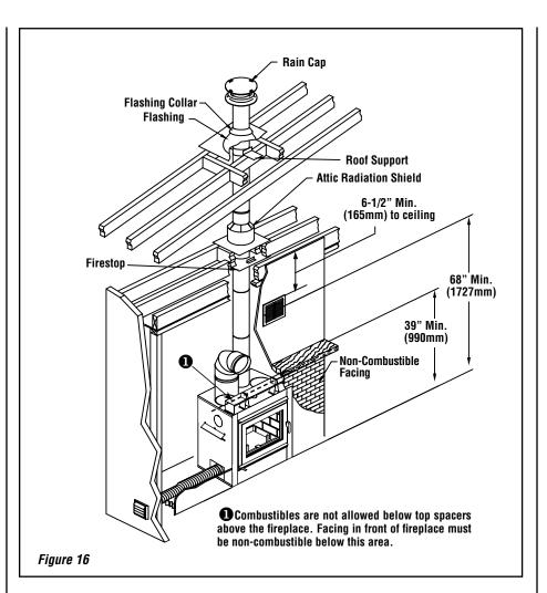
The duct system must be installed respecting the following:
