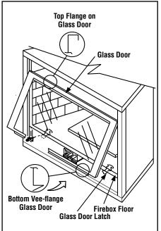
Figure 6 - INSTALLING GLASS DOOR
