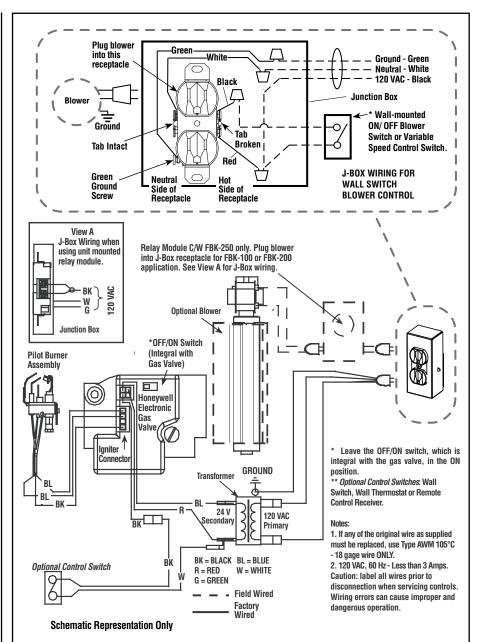
Electronic Wiring Diagram (Honeywell) Showing Blower Wiring for Optional FBK-100, FBK-200 & FBK-250 Kits Figure 17
