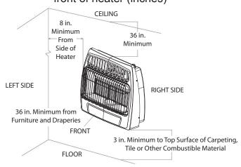
Fig. 2 - Mounting clearances as viewed from front of heater (inches)
