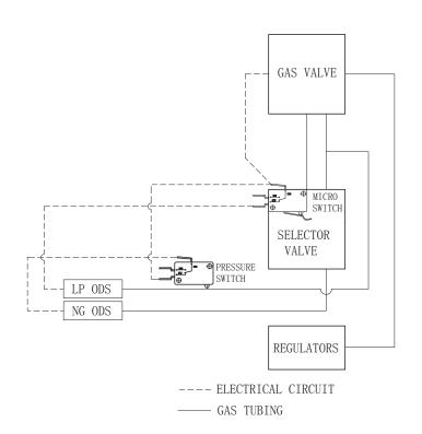
**NOTE:** Pressure Switch opens at 8.0" WC manifold pressure.
