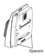
Fig. 19b - Mounting Heater Onto Mounting Bracket
