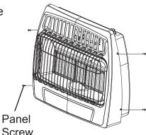
Fig. 30 - Front Panel Removal
