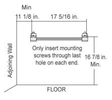
Attaching to Expansion Bracket Method For attaching mounting bracket to hollow walls (wall areas between studs) or solid walls (concrete or masonry):
