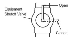
Fig. 21 - Equipment Shut -off Valve
