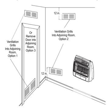
Fig. 2 - Ventilation Air from Outdoors
