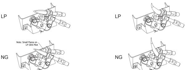
Fig. 27 - Incorrect Pilot Flame Pattern
