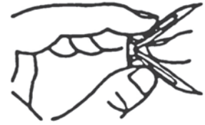
Fig. 17 - Folding the Expansion Bracket
